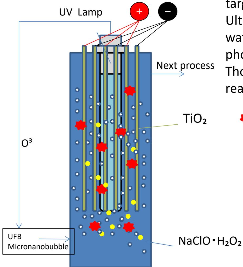
AOP<sup>+</sup> has been designed to generate active free radicals ( $\cdot\text{OH}$ ) and attack targets effectively as Ultra Fine Bubble put pressure to the water and electricity excite reactions of photocatalyst. Those are the reason why chemical reaction are much improved.
